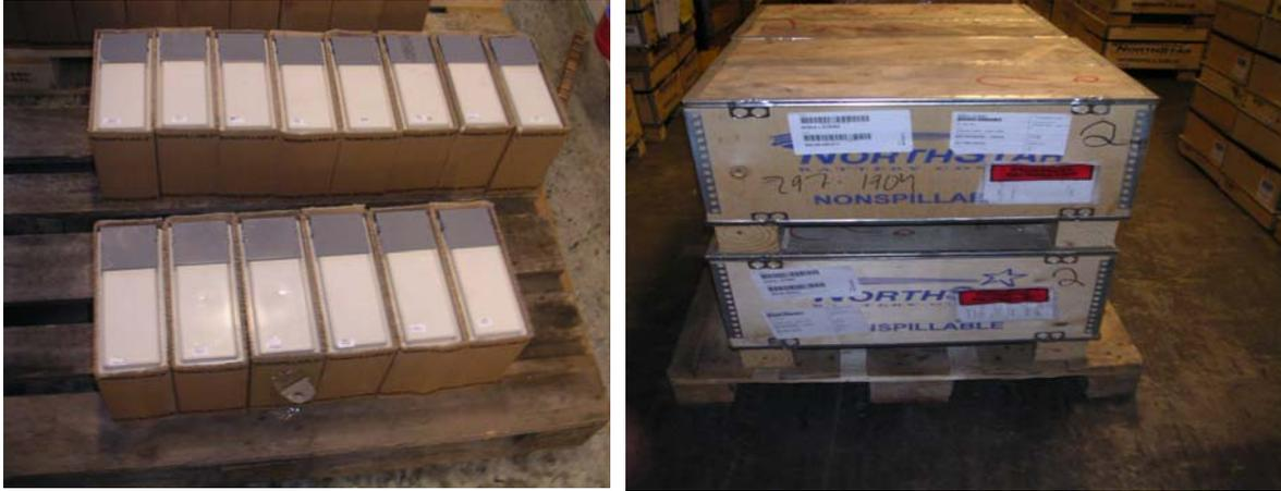
Figure 2 Different ways to correctly store batteries
